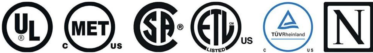
Figure 1. Examples of NRTL listing marks, a required feature on every device plugged into AC power in a workplace.
