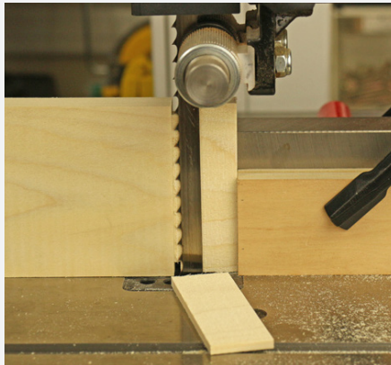
A typical band saw operation that requires an operator to retrieve the material while the machine may still be coasting.
