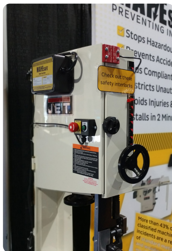
The Power Tool Brake installed on a 1.5HP bandsaw with door interlocks.
