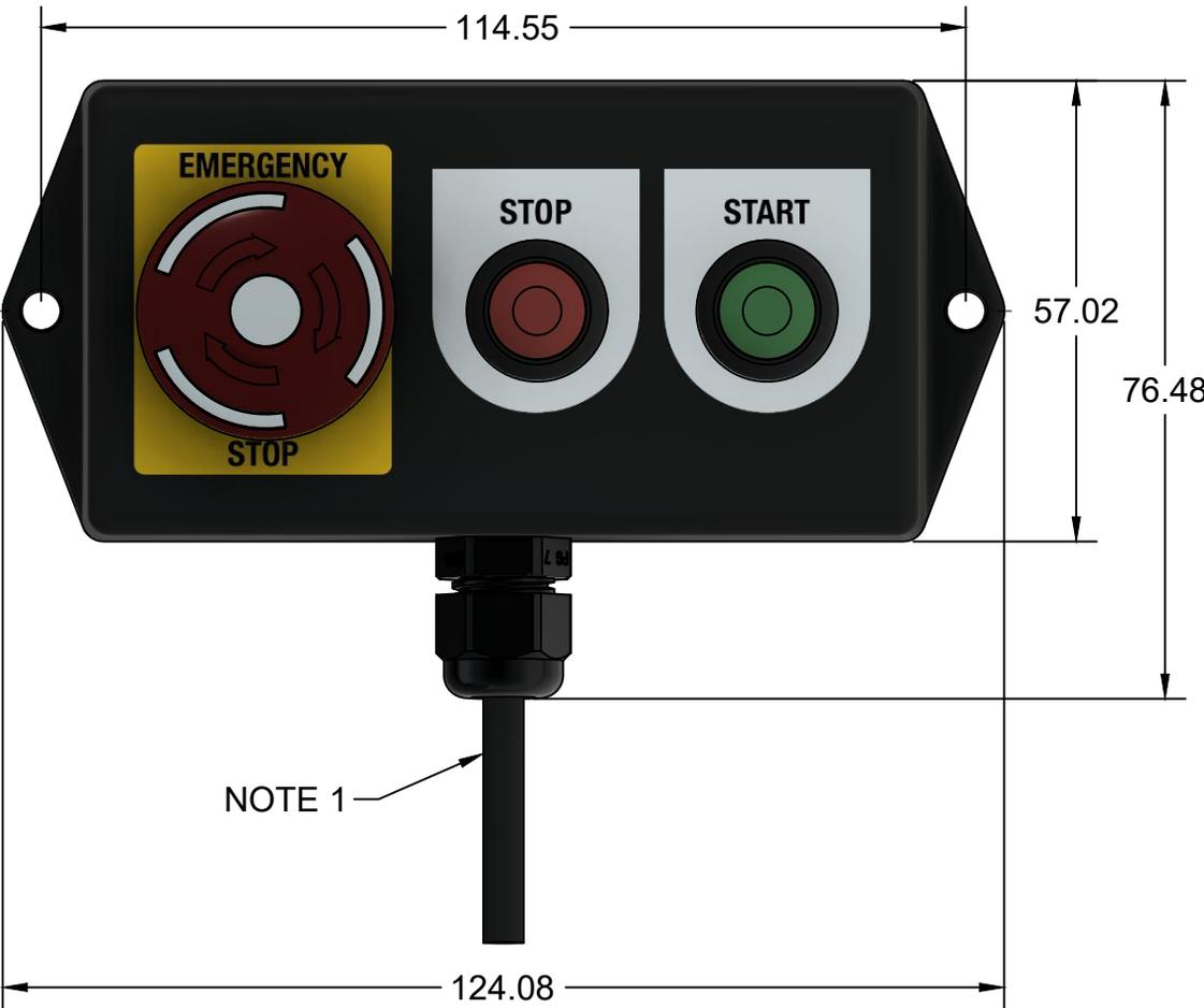
NOTE 1: PROVIDE ADEQUATE SPACE BELOW CONTROL PANEL FOR A MINIMUM CABLE BEND RADIUS OF 25MM. ALTERNATE CABLE EXIT DIRECTIONS AVAILABLE BY SPECIAL ORDER.
